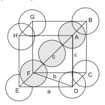
Fig. 6.19. Body centred cubic until cell.
