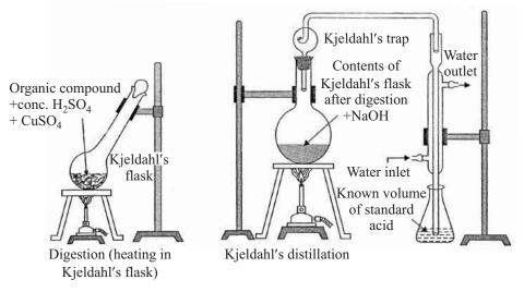
Fig. 23.5 Kjeldahl's method
