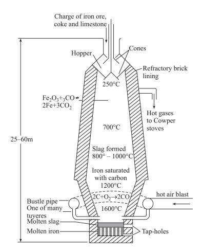
The energy and reducing agent required for the smelting of iron are obtained by the combustion of coke, the temperature of the charge increasing steadily as it falls through the ascending combustion gases:
