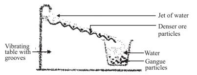
Fig. 16.3: Gravity Separation (Hydraulic Washing)
