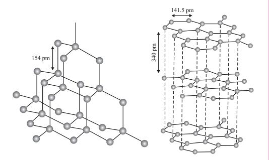
Fig. 19.5: Structure of diamond
