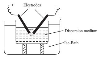
Fig. 8.2: Preparation of colloidal solution by Bredig's Arc Method
