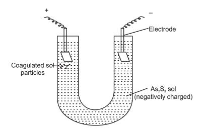
Fig. 8.7: A set up for Electrophoresis
