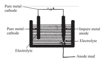
Fig. 16.8: Electrolytic Refining
