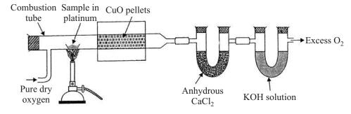
Fig. 23.2 Estimation of carbon and hydrogen
