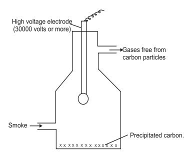
Fig.8.8: Cottrell smoke precipitator
