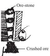
Fig. 16.1: Jaw Crusher
