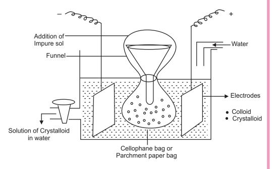
Fig. 8.4: Electrodialysis
