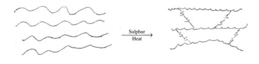
Fig. 31.4: Process of vulcanization of rubber
