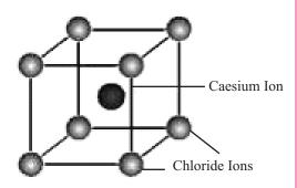
Fig. 6.21: Caesium chloride structure
