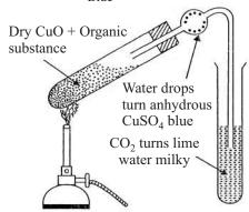
Fig. 23.1 Detection of carbon and hydrogen
