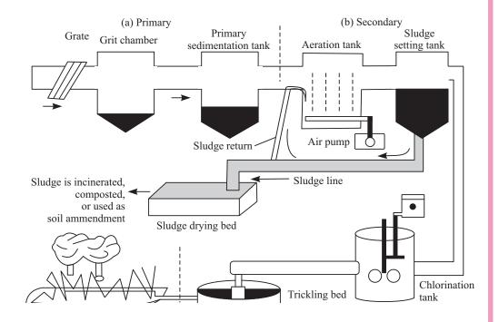
Fig. 32.8: Treatment process of sewage
