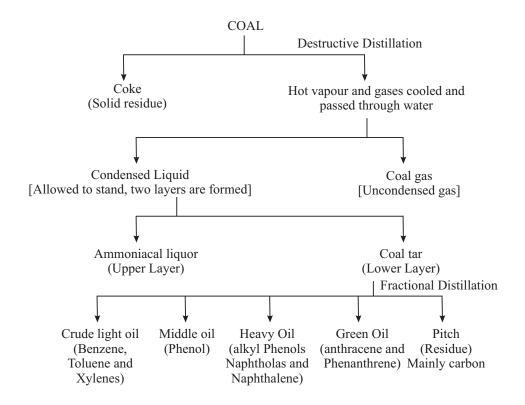
Fig. 24.1: Destructive Distillation of coal
