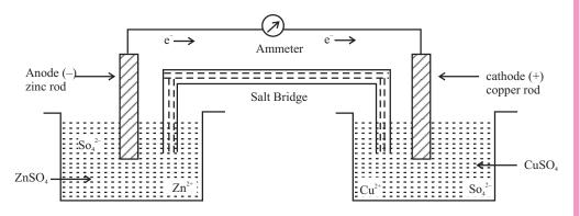
Fig. 13.6: Daniell cell having zinc and copper electrodes
