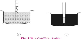
Fig. 5.21: Capillary Action
